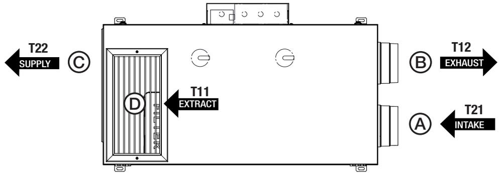
Fig. 7.a Temperature probes
