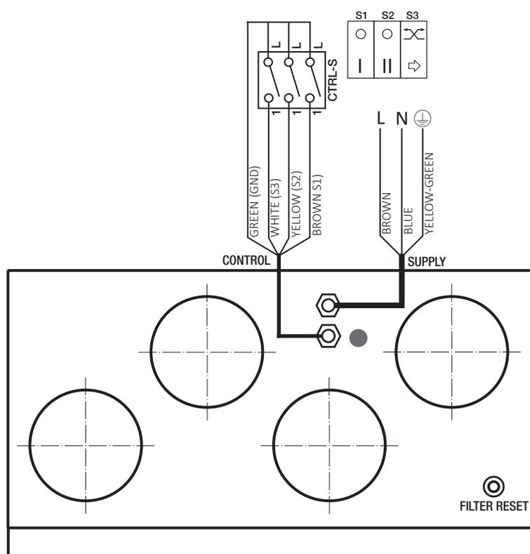
Fig. 5.j Electric connections
