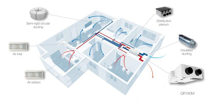
How it works: a continuous running heat recovery unit (QR180M) transfers heat from humid air extracted from wet rooms to warm incoming fresh air which is ducted to habitable rooms. Thanks to the easy-to-fit air distribution system each single ambient can be properly ventilate: the boost function enables rapid extract of increased moisture or pollutant levels. It also provides discrete installation and very quite operation.
