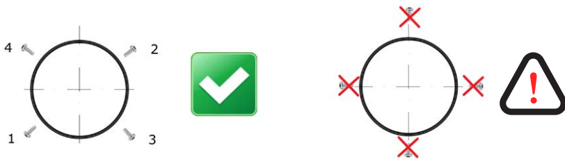
Fig. 4.1. Connecting the air ducts and fittings to the humidifier (it is forbidden to screw the self-tapping screws on the horizontal and vertical axes – this may
